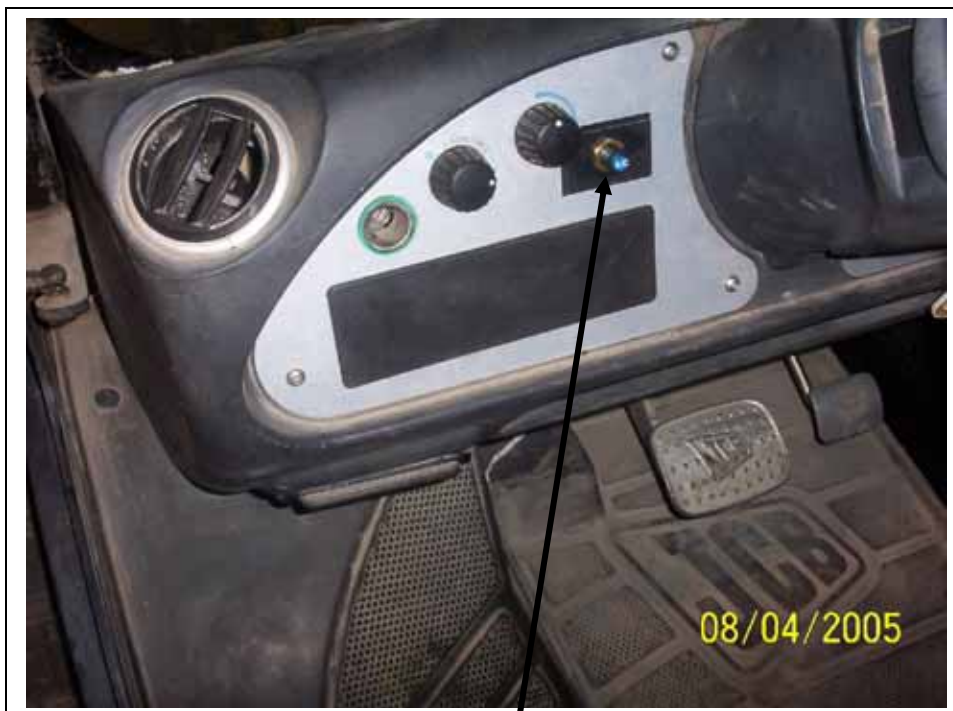
A/C switch installed.
