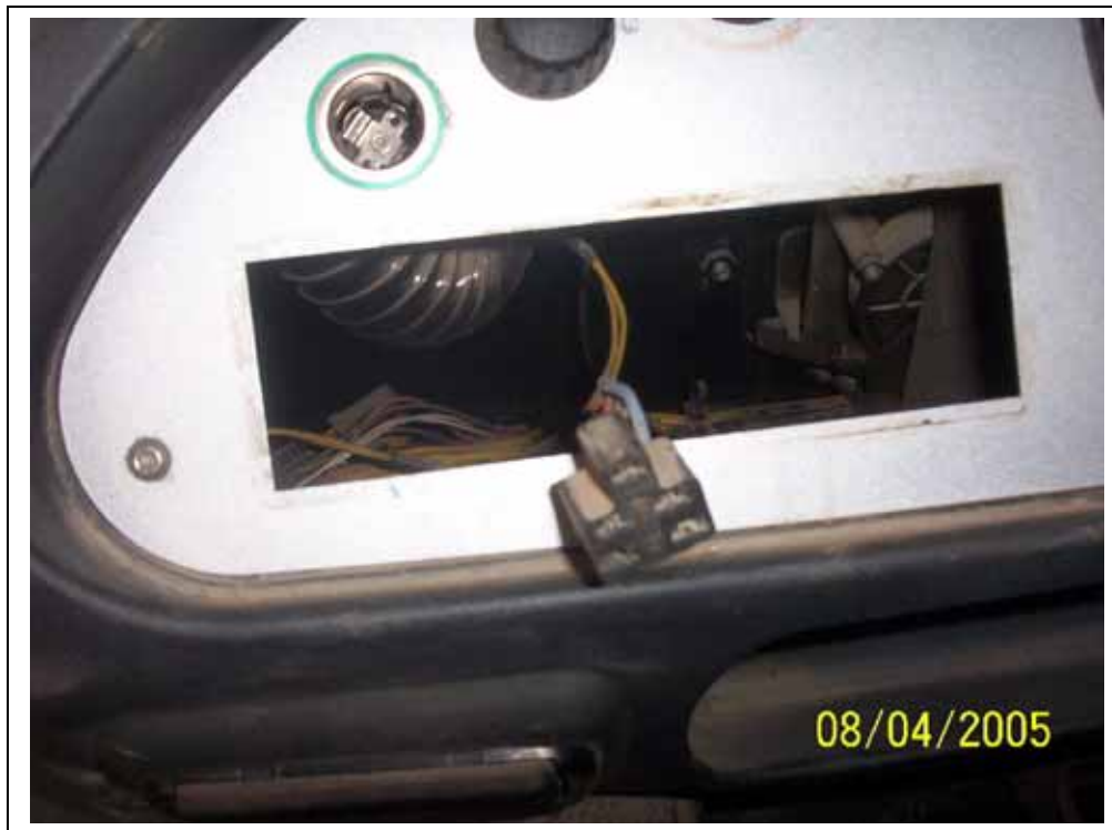
Remove left front dash panel
