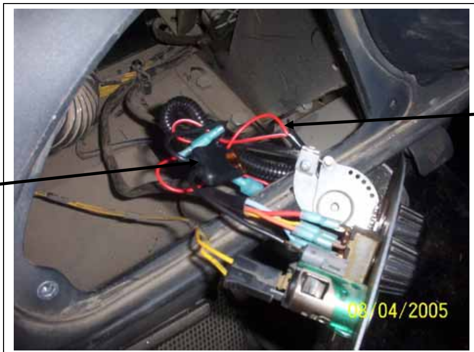
A/C on-off switch installed with 7.5 amp fuse and holder.
