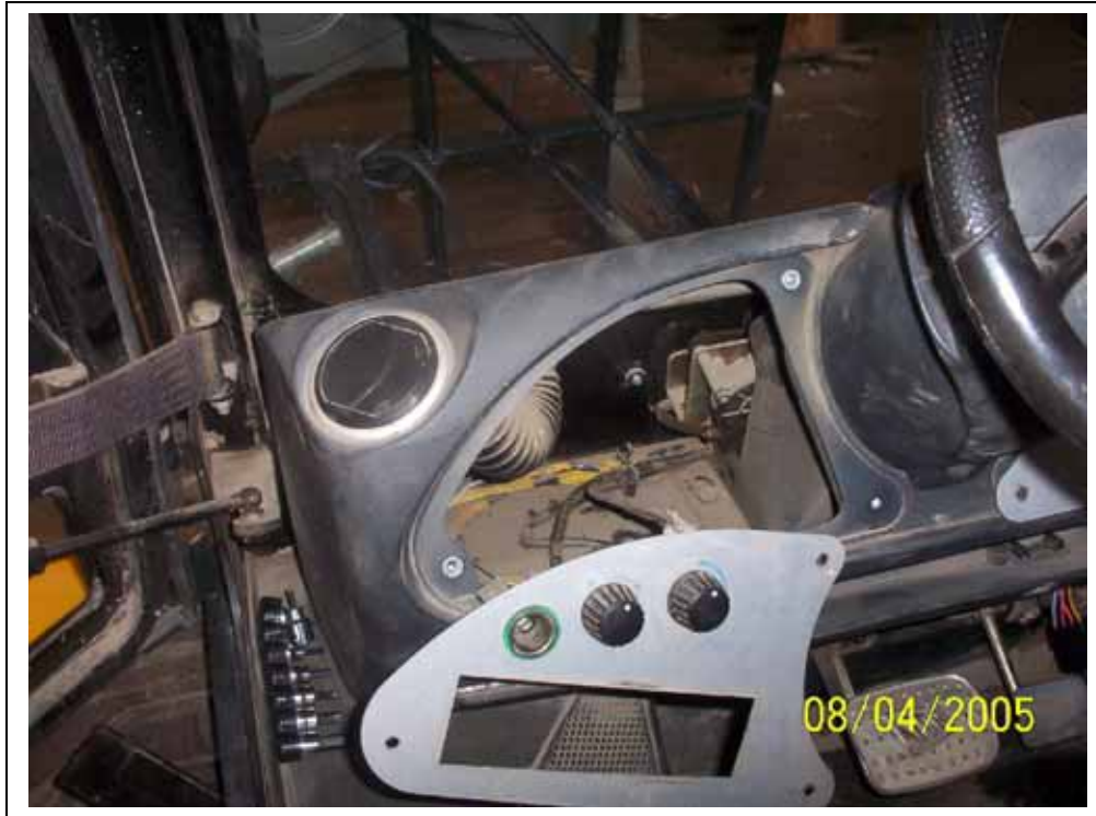
Remove left front dash panel
