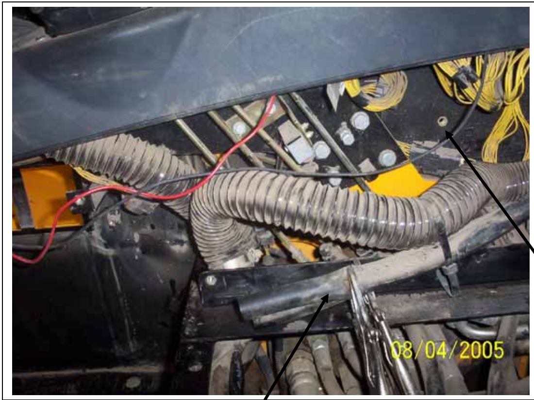
Heater lines clamped off and flex duct removed
