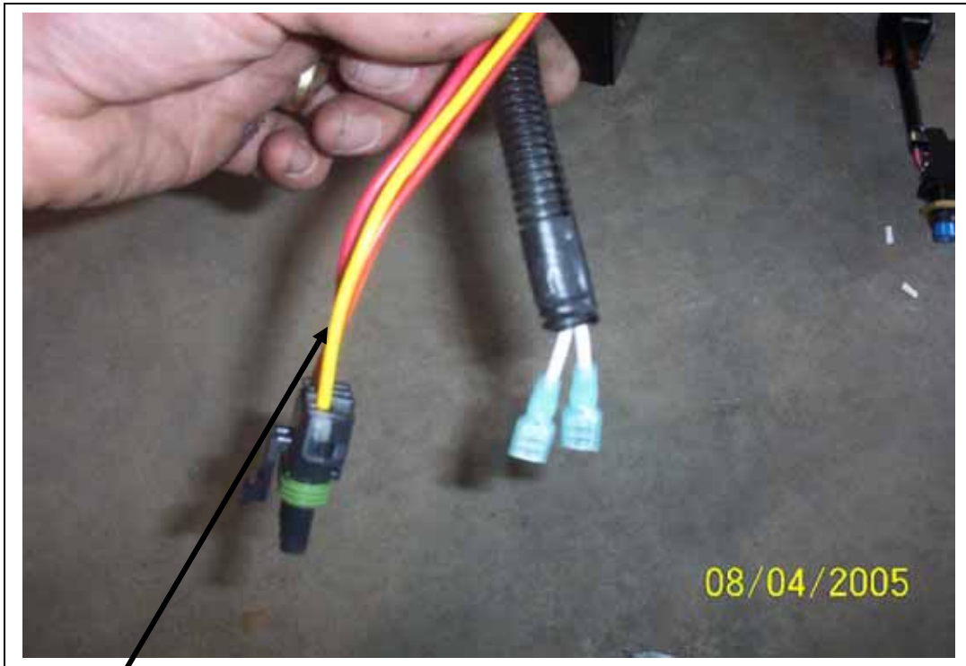
Thermostat wires. In from relay and the out to binary switch at
