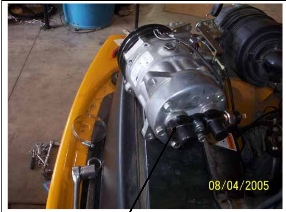
Install rear pad onto compressor. Smaller fitting on discharge side, larger fitting on suction side as shown.
